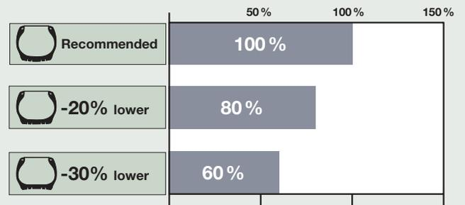
The proper inflation pressure is essential for the correct performance of all kinds of tyre. YOKOHAMA recommends proper maintenance and utilisation of a calibrated gauge / inflation pressure sticker or TPMS.
